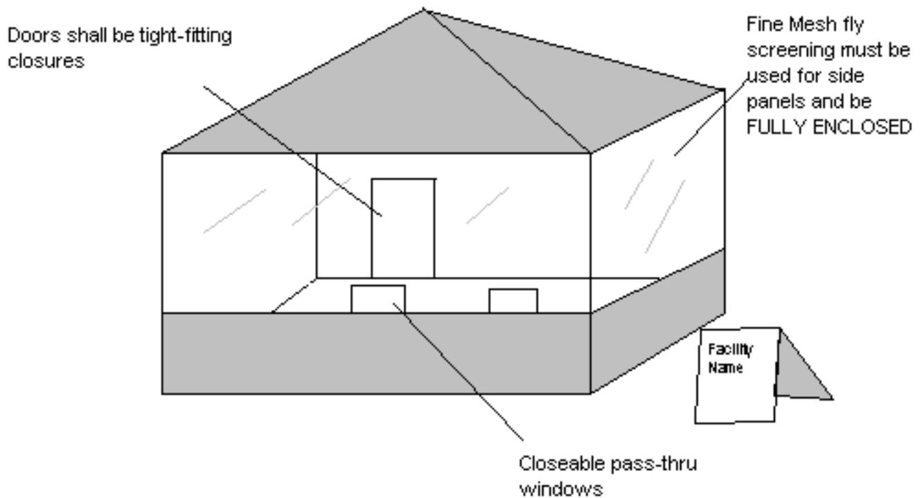
**NOTE:** Roof and side panels may be plywood, fiberglass, plastic, or canvas board with wood or metal framing.
